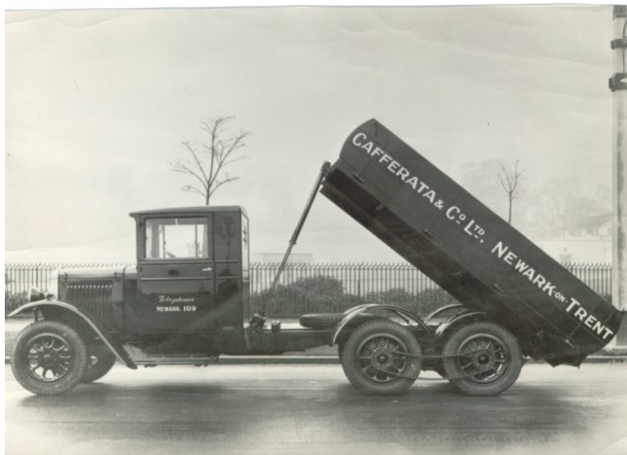
A truck of the inter-war years : the chain drive wasn't effective in muddy quarries
